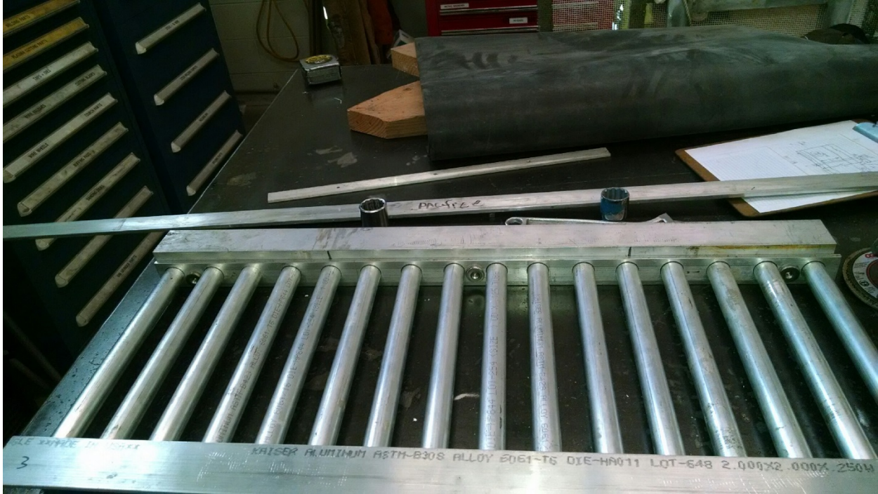
Photo 3. Fabrication of replacement bars for false weir.
